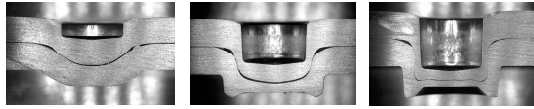
Fig. 1. Plastic deformation of the upper and lower sheet in the mechanical clinching process.
